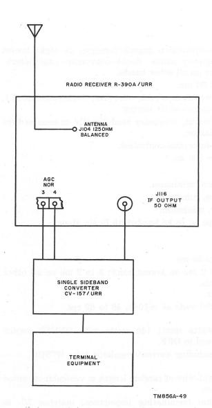
Figure 4. Single-sideband radioteletype system, block diagram.
