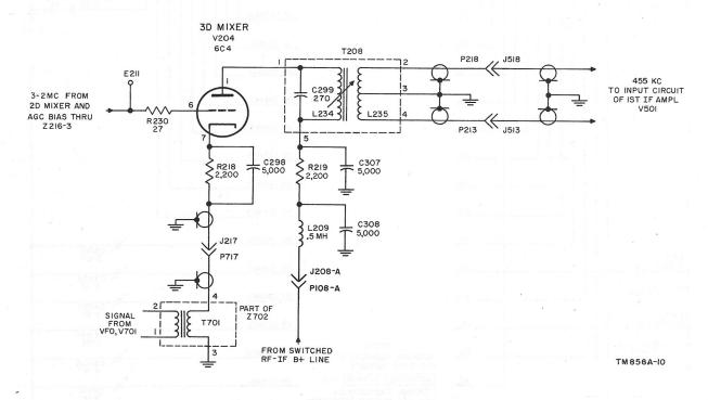
Figure 27. Third mixer V204, schematic diagram.
