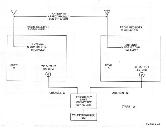
Figure 3. Two space-diversity radioteletype systems, block diagram.
