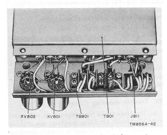
Figure 72. Power-supply subchassis, bottom view.
