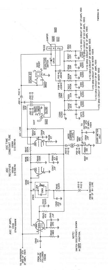
Figure 38. Agc circuit, schematic diagram.
