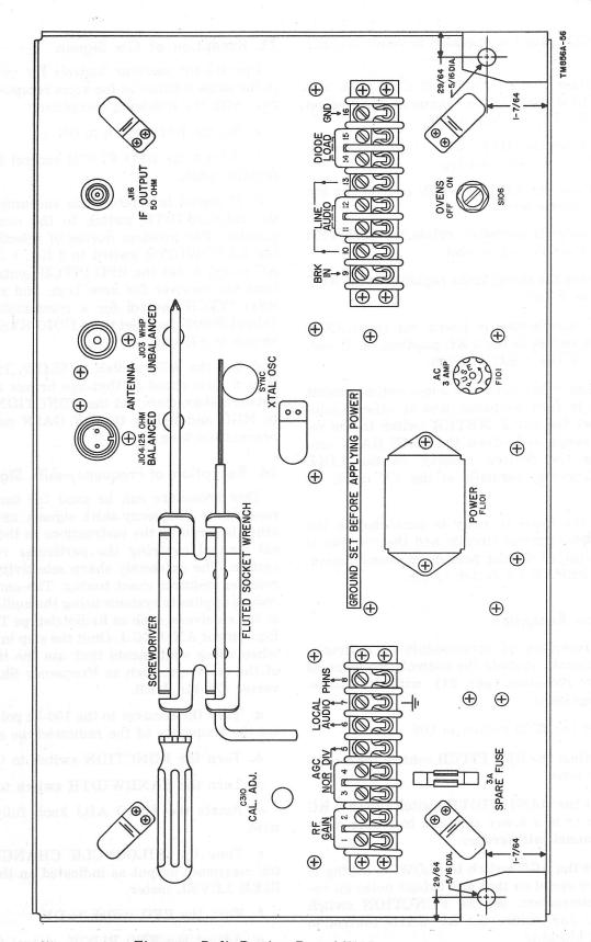
Figure 12. Radio Receiver R-390A/URR, rear panel.
