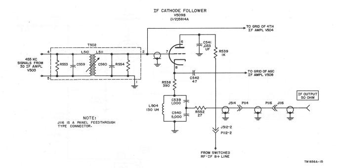
Figure 37. If cathode follower V509B, schematic diagram.
