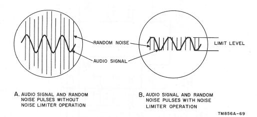
Figure 35. Typical oscilloscope presentation of limiter operation.
