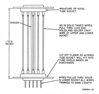
Figure 54. Fabrication of tube test point adapters.
