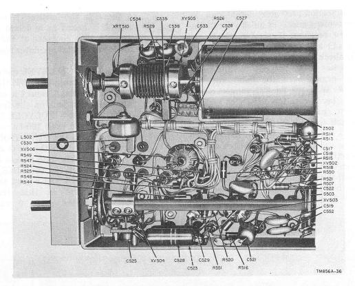
Figure 66. If subchassis, bottom view, front section.
