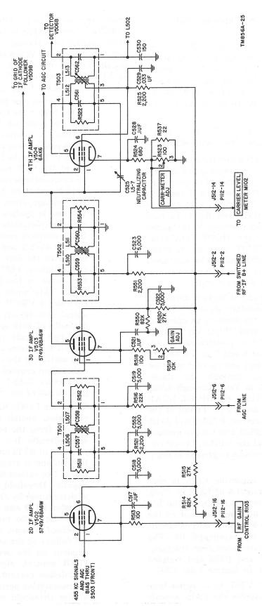
Figure 33. Second, third, and fourth if amplifiers V502 through V504, schematic diagram.
