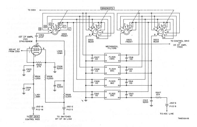
Figure 30. First if amplifier V501, schematic diagram.
