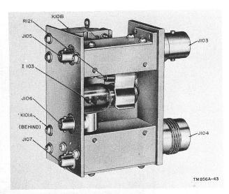
Figure 73. Antenna relay assembly, internal view.
