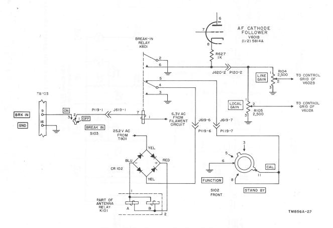
Figure 45. Break-in circuit, schematic diagram.
