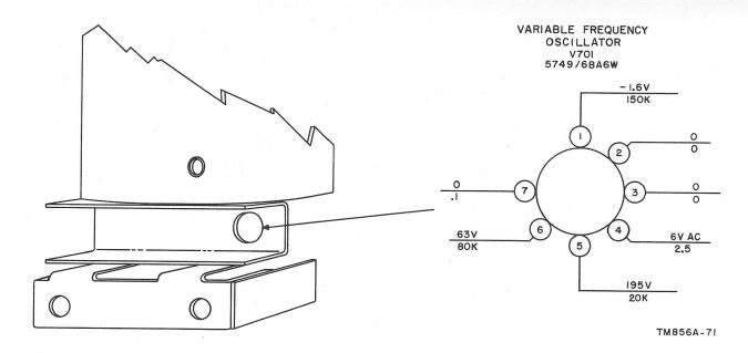
Figure 78. Vfo subchassis, voltage and resistance diagram.
