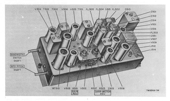
Figure 64. If subchassis, top view.
