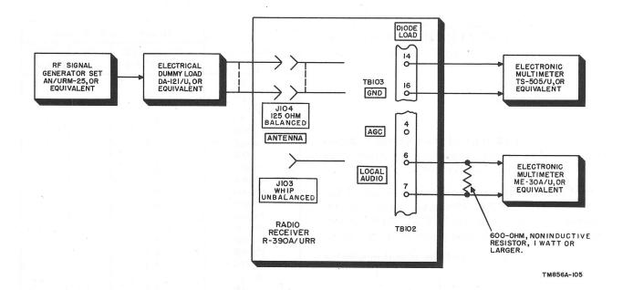
Figure 99. Sensitivity and over-all gain, test setup.
