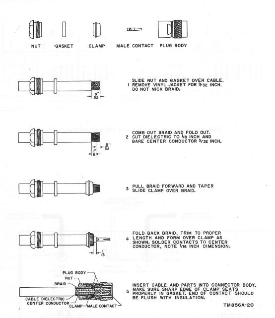
Figure 9. Assembly of Connector Plug UG-573/U to coaxial cable.
