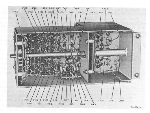
Figure 62. Crystal-oscillator subchassis, bottom view.
