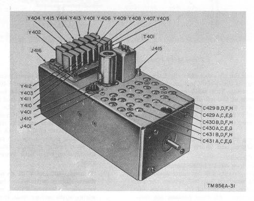
Figure 61. Crystal-oscillator subchassis, top view.
