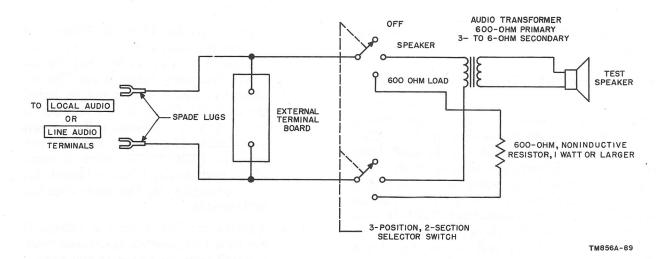
Figure 55. Test-speaker assembly fabrication.
