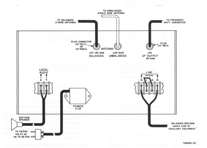
Figure 8. Radio Receiver R-390A/URR, cording diagram.
