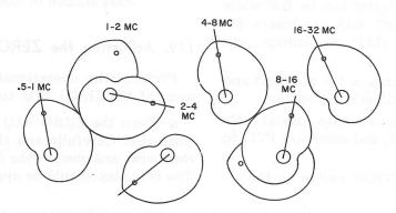
CAM POSITIONS VIEWED FROM REAR WITH 2 REAR PLATES REMOVED IN 7 +000 MC POSITION
