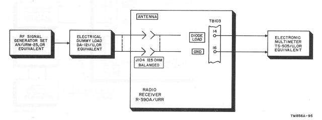
Figure 98. Over-all selectivity test setup.
