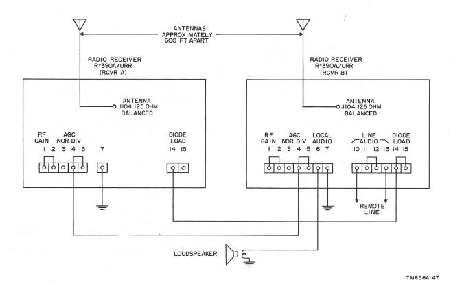
Figure 2. Space-diversity receiving system, block diagram.
