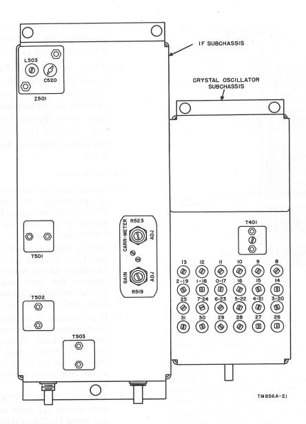
Figure 90. Crystal-oscillator and if subchassis alignment points.
