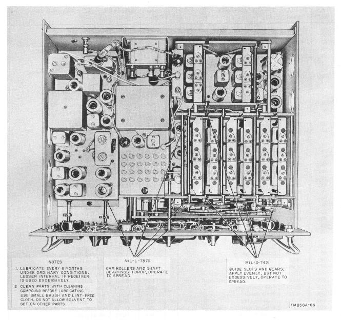
Figure 85. Radio Receiver R-390A/URR, Lubrication points.
