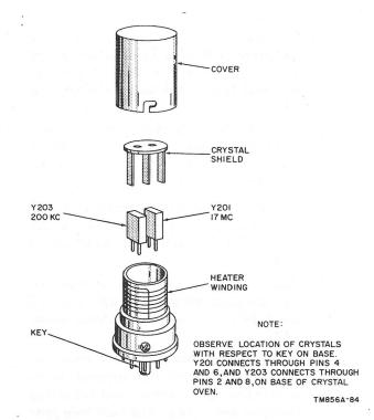
Figure 83. Location of crystals Y201 and Y203.
