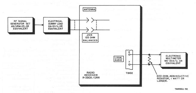
Figure 94. Receiver audio test setup.
