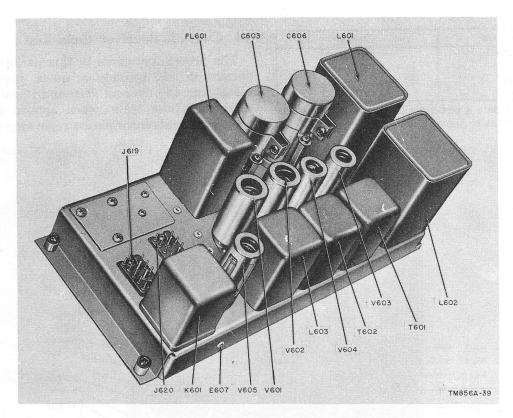
Figure 69. Af subchassis, top view.
