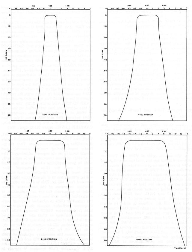
Figure 32. Band pass of mechanical filters.
