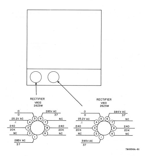
Figure 80. Power-supply subchassis, voltage and resistance diagram.
