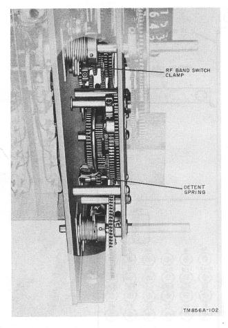
Figure 88. Location of rf band switch shaft clamp and detent spring.
