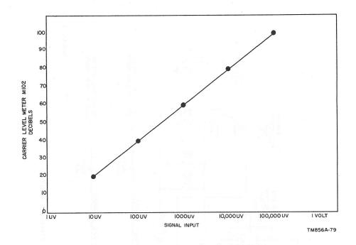
Figure 41. CARRIER LEVEL meter reading versus signal input.
