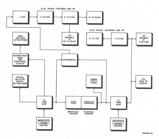
Fig. 49. Tuning system, mechanical, block diagram.
