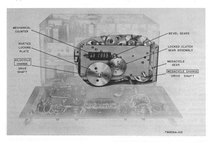
Figure 86. Rf gear train assembly, location of parts.
