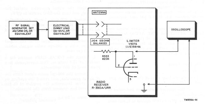
Figure 96. Limiter clipping level test setup.
