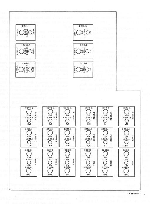
Figure 91. Rf and variable if alignment points.
