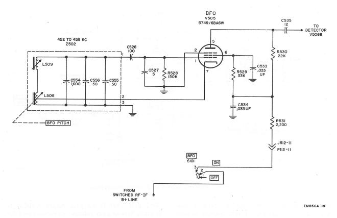
Figure 36. Beat-frequency oscillator V505, schematic diagram.
