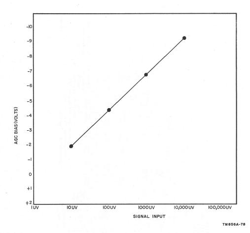
Figure 39. Imput signal versus developed agc bias.
