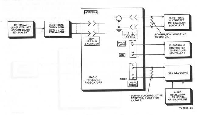
Figure 97. Bfo calibration and if output test setup.
