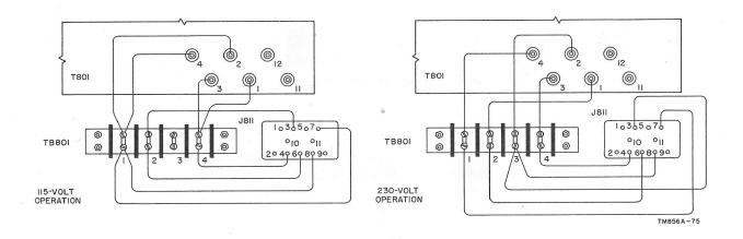
Figure 7. Connections for 115-volt or 230-volt operation.
