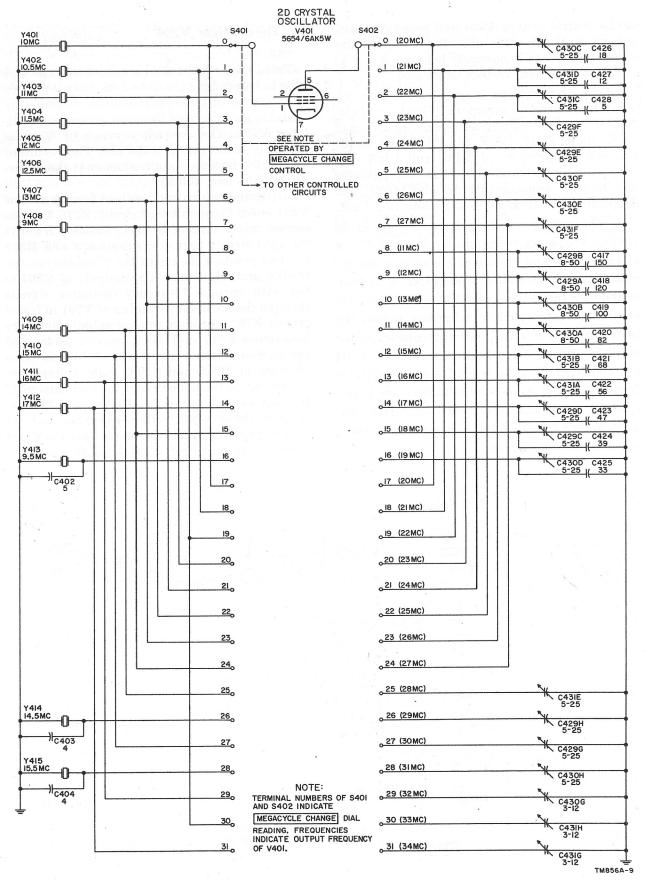
Figure 26. Second crystal oscillator V401, crystal and plate switching, schematic diagram.
