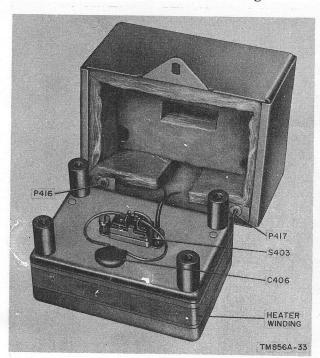
Figure 63. Crystal-oscillator subchassis, internal view of crystal oven.
