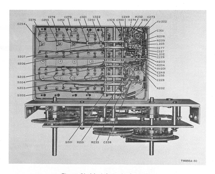
Figure 59. Rf subchassis, bottom view, front section.
