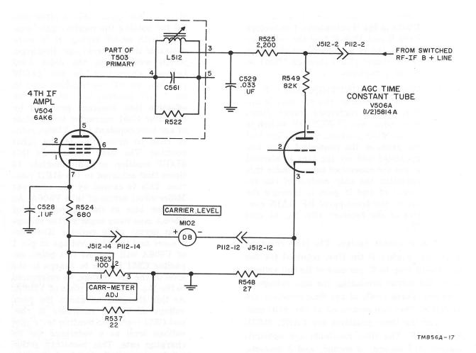
Figure 40. CARRIER LEVEL meter circuit, simplified schematic diagram.
