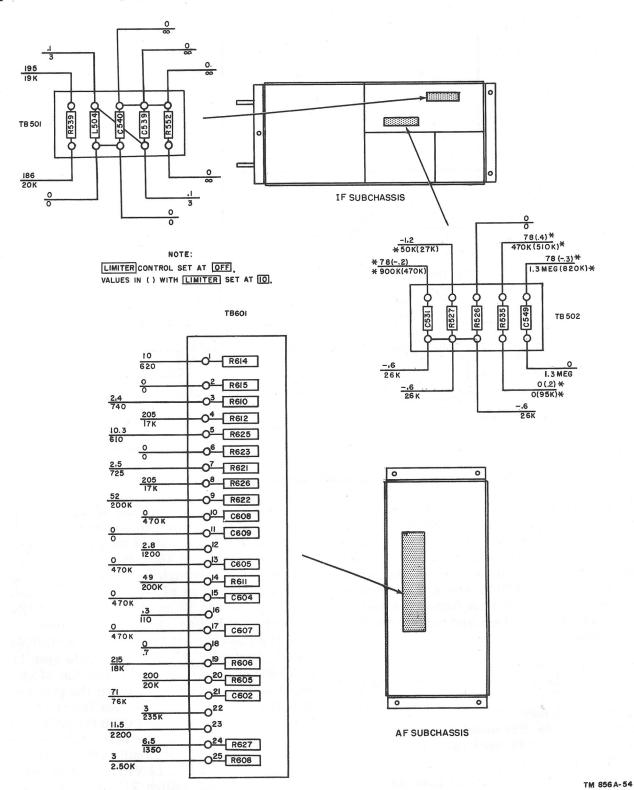
Figure 81. If and af subchassis resistor and capacitor boards, voltage and resistance diagram.
