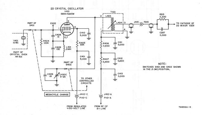
Figure 25. Second crystal oscillator V401, schematic diagram.
