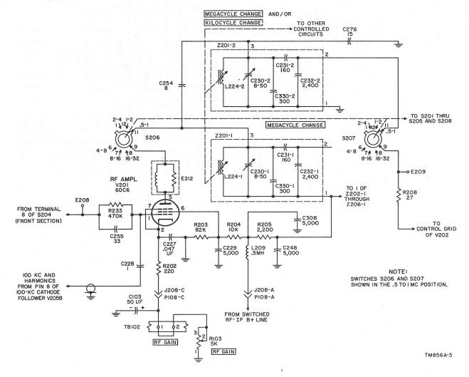
Figure 20. Rf amplifier V201, schematic diagram.
