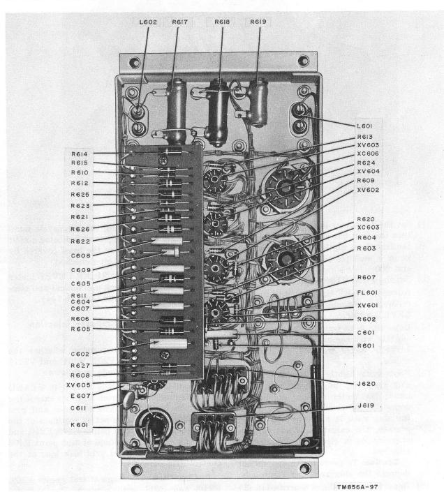
Figure 70. Af subchassis, bottom view.
