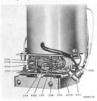
Figure 68. Vfo subchassis, bottom view.
