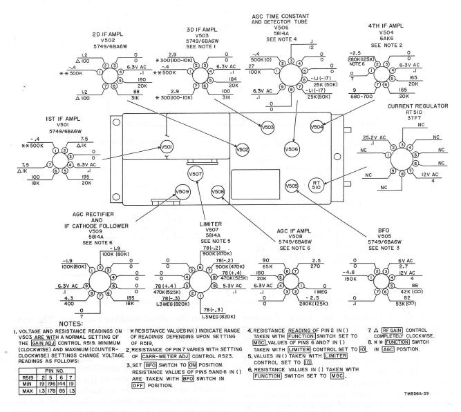
Figure 77. If subchassis, voltage and resistance diagram.
