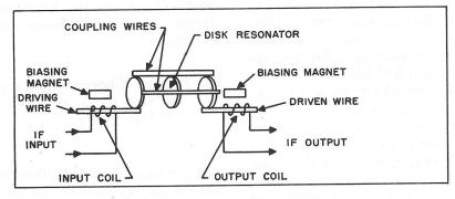
A. COMPONENTS OF A MECHANICAL FILTER
