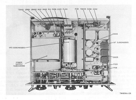
Figure 57. Radio Receiver R-390A/URR, bottom view.
