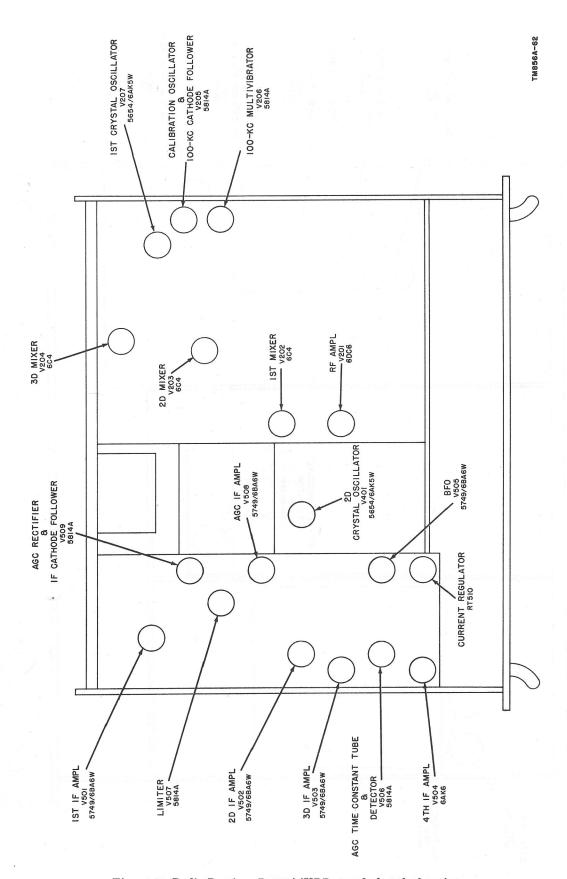
Figure 15. Radio Receiver R-390A/URR, top deck, tube location.
