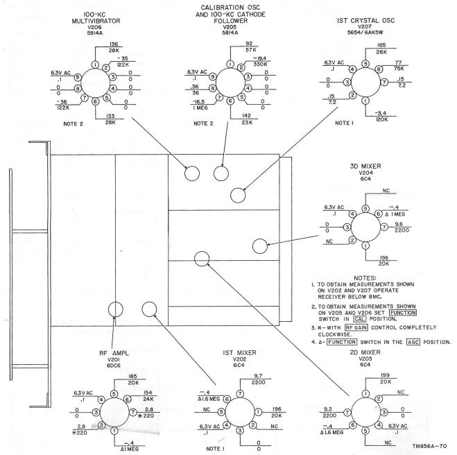
Figure 75. Rf subchassis, voltage and resistance diagram.
