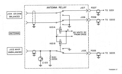
Figure 18. Antenna circuit, schematic diagram.
